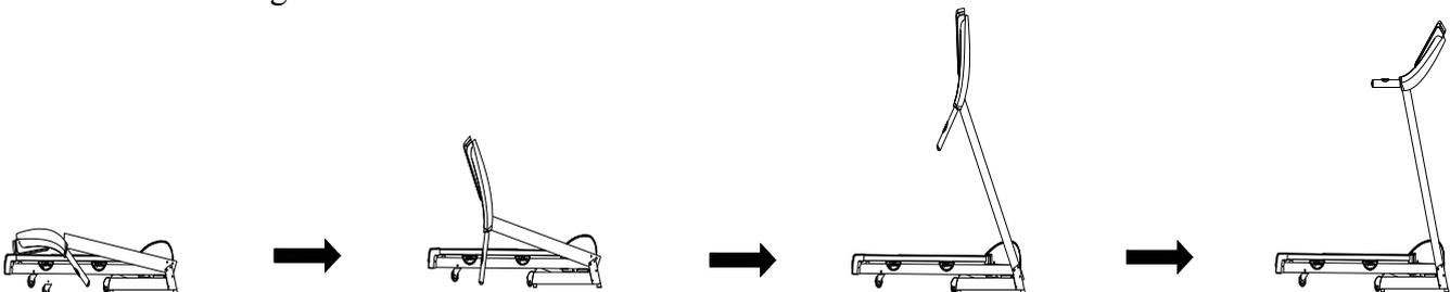
**STEP 2:** According to the picture to tighten the bolt M8\*45 (D16) , M8\*15 (D13) and inner washer (D17) . Then Locked with M8\*15(D13) and inner washer (D17).
