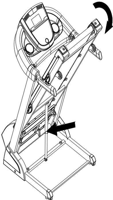
Push the safety sleeve with your foot lightly and pull down the machine at the same time as the arrow direction. Then the machine will fall down smoothly.
